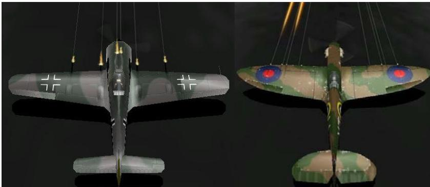
Wing mounted weapons configurations were much more variable in layout because of a number of factors. Weapons placed near the fuselage often had problems with having to fire through the propeller arc. This required those guns to be synchronized so that they didn't hit the propeller and thus took a penalty in their
